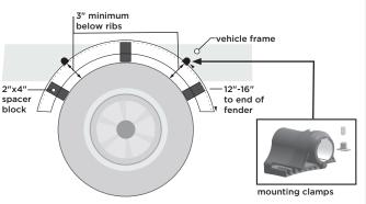
Once the position of the mounting tube is chosen, slide the other mounting clamp onto the tube, making sure that
