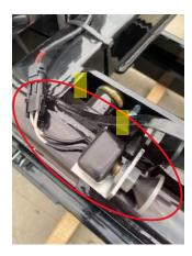
Step 3) Use a jumper wire to complete the circuit to winch stop switch's connector that goes to the winch.
